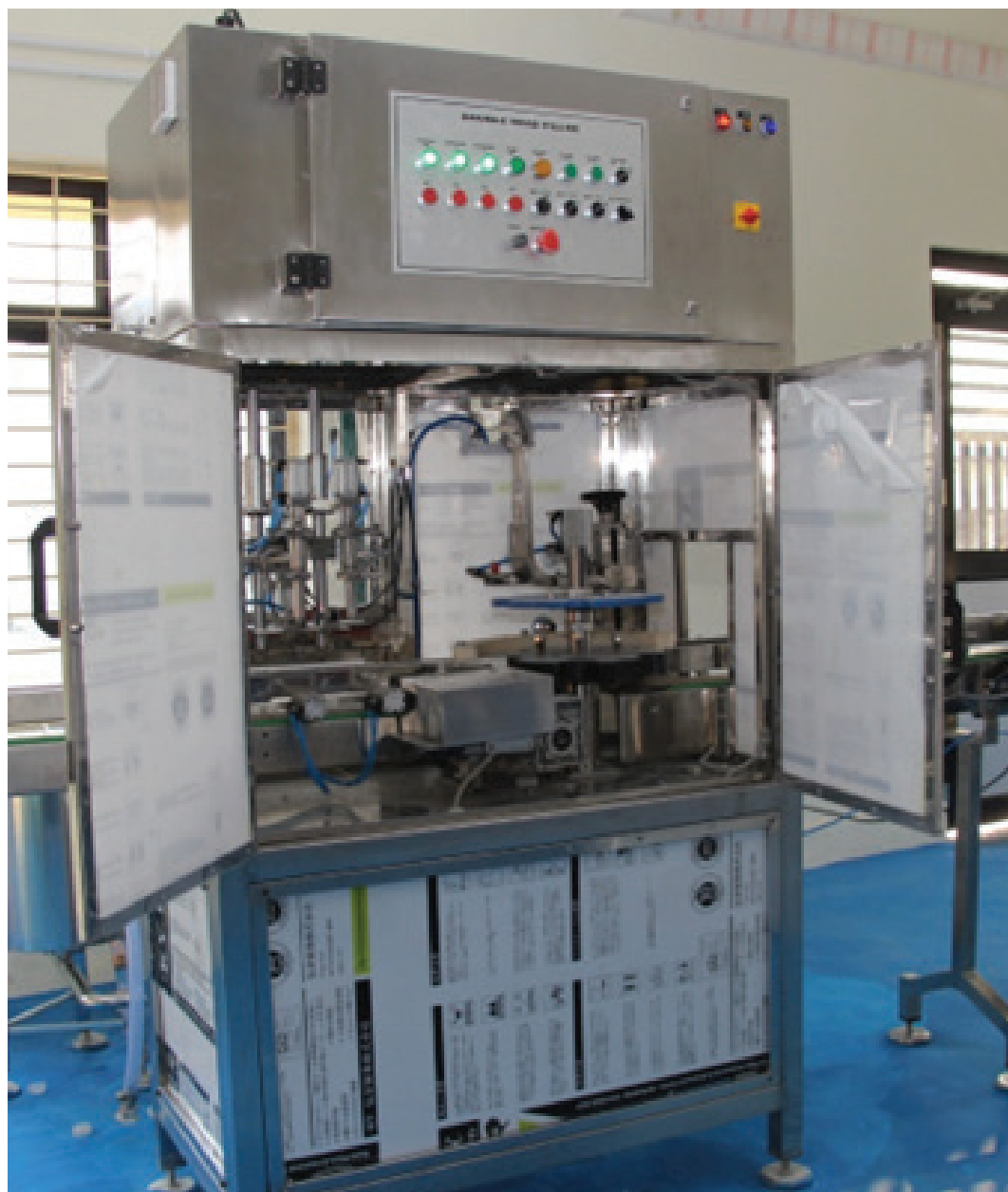
Fig. 7 Automatic bottle filling and capping machine with attached hopper to fill formulations
