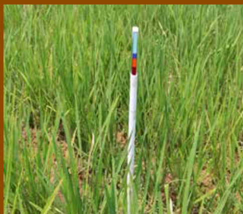
Fig. 2.7. Customized colour coded tensiometer for scheduling irrigation in rice
