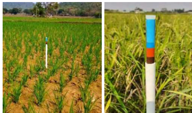
Fig. 4. Representative picture of Customized Color Coded Tensiometer in rice field.
