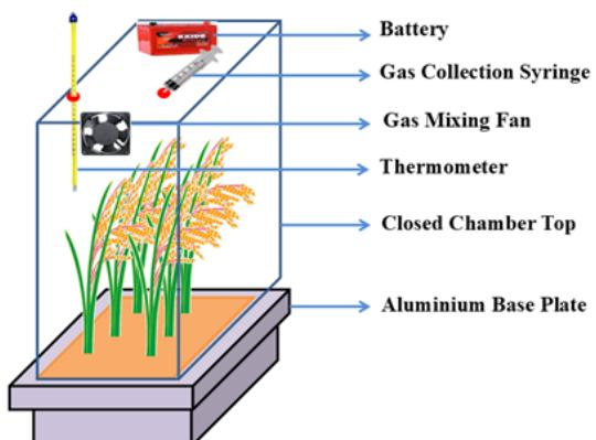
Standard dimensions are approximately 50 × 30 × 100 cm, typically made from 6-mm thick acrylic sheets, especially for use in rice paddies.
