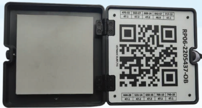
Fig. 7 White Calibration panel
