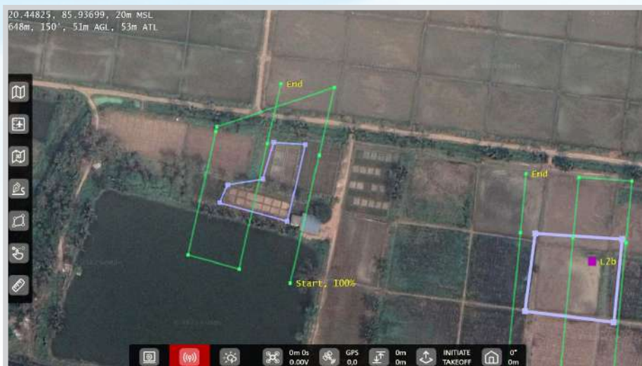
Fig. 2 Generation of mapping plan using blue fire touch software
