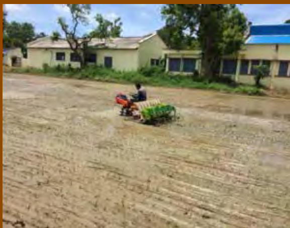
Fig. 2.12. Urea briquette applicator attachment for mechanical rice transplanter
